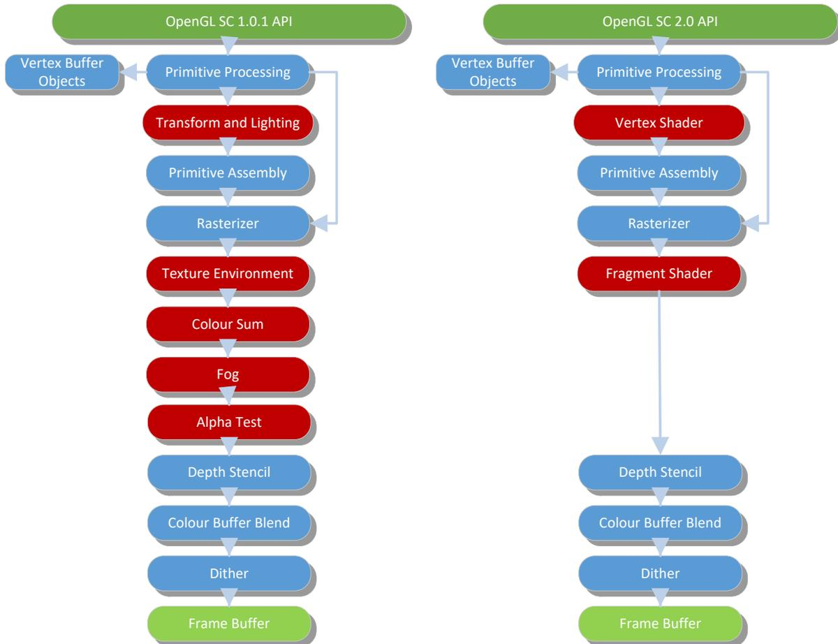
Figure 2: Differences Between Fixed Graphics Pipeline and Programmable Graphics Pipeline
